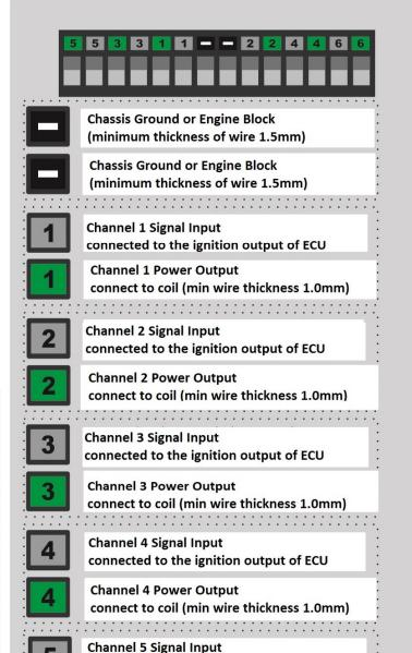
connected to the ignition output of ECU
