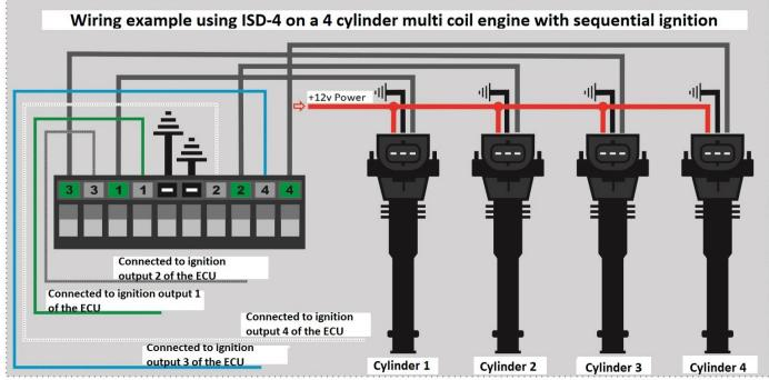
Never connect ISD ground to battery, **ALWAYS** use ground on chassis or engine block. It is very important that the negatives (-ve) have **good electrical contact** with the chassis/block. Set the module ignition output type to ISD
