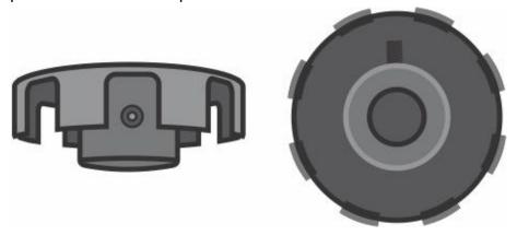
5. Alignment of the table relative to the sensor is very important. This joint is responsible for engine ignition point and fuel injection in the right moment, so is necessary that this "window" is on average 1mm greater than one of the other sides for the module has TDC reference of cylinder 01. (Choose the side that will pass through the sensor to remove material).
