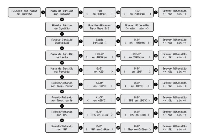
In the setting of ignition maps, the user has total control of the engine point, as well the creation of point main map and ignition corrections by engine temperature, air, TPS, and Map. Also is possible to do the advancement or retardment in every map by making a quick injection adjustmentIn addition, the idle speed map adjustment allows a more stable control having a specific map for this function.
