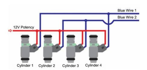
Blue Output 1 – Injector A-1 – Cylinder 01 and 04 Blue Output 2 – Injector A-2 – Cylinder 02 and 03
