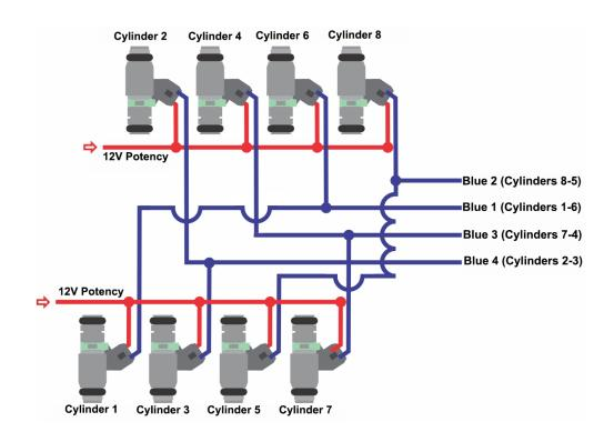
Blue Output 1 - Injector A-1 - Cylinder 01 and 06
