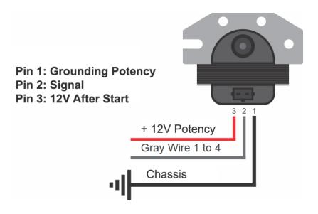
**Tip:** The higher the number of cylinders, the shorter the time for the coil to charge, discharge and rest, then monitor the temperature of the coil's ignition module and if it is overheating, quickly reduce the Dwell.
