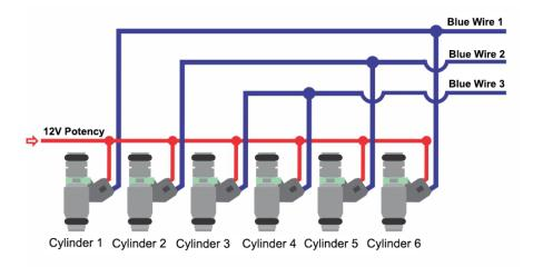
Blue Output 1 - Injector A-1 - Cylinder 01 and 06
