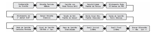
The menu above is responsible for the main ignition configuration where we will define the number of cylinders and the mode of rotation capture. This is undoubtedly the most important configuration of the module. If it is not set correctly the engine will not work and may still cause serious damage to the engine or its components.
