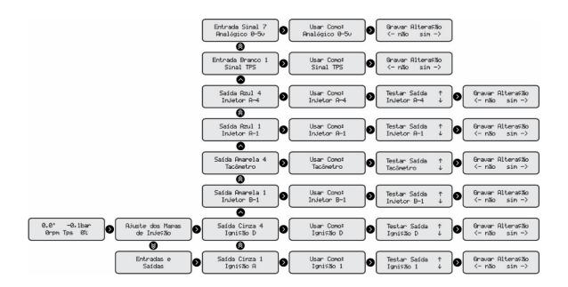
The "Test Output" screen is a function that allows you to test the module channel. When clicking the up or down button, the module sends pulses when the output is configured as a fuel injector or coil, or approximately 3s negative signal when configured with another function.
