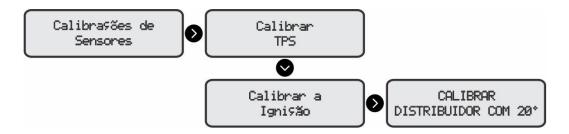
**Note:** When configured as a distributor, you should calibrate the window size before calibrating the ignition; if this calibration is not made, may happen a divergence at the ignition point.
