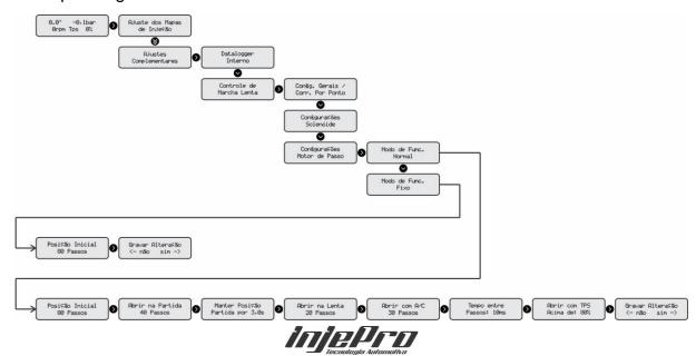
**Normal Mode** – Operate forward or backward with up to 260 steps. **Fixed Mode** – Once calibrated, the piston is fixed in the configured position.
