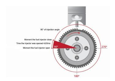
In the second example, when configured "Pulse End" and Injection Angle programmed to 90° the S4500 starts the pulse 4.63ms before the 90° TDC, so the fuel injector will finish its cycle and then the injection angle begins. This mode is the most used and most accurate too.
