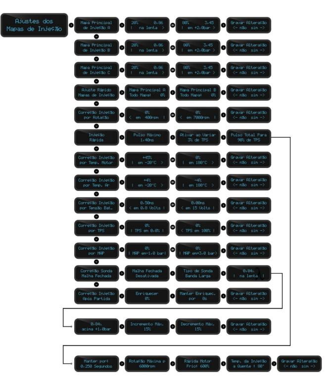
This menu above is responsible for all fuel injection control such as Map Benching A, Benching B, and Benching C or Map A / B or A / B / C when semi-sequential to 4 or 6 cylinders.
