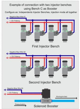
If you choose to install the S3000 in a 6 cylinder engine it is also possible to make it semisequential using the 3 injector outputs and connect them on their respective even cylinders. The arrangement would stay as follows: Bench A - Cylinders 1-6, Bench B - Cylinders 2-5 and Bench C -Cylinders 3-4.
