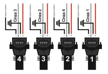
Tip for timing positive of fuel injectors and coils.
