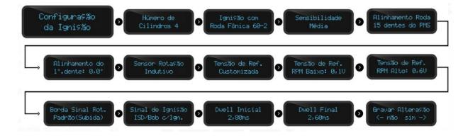
The menu above is responsible for the main ignition configuration where we will define the number of cylinders and the mode of rotation capture. This is undoubtedly the most important configuration of the module. If it is not set correctly the engine will not work and may still cause serious damage to the engine or its components.
