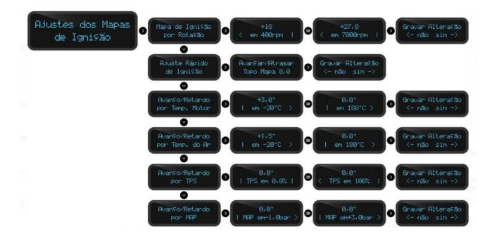
In the setting of ignition maps, the user has total control of the engine point, as well the creation of point main map and ignition corrections by engine temperature, air, TPS, and Map. Also is possible to do the advancement or retardment in every map by making a quick injection adjustment.
