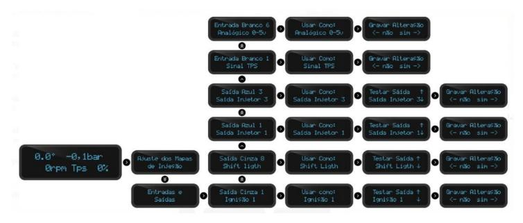
The "Test Output" screen is a function that allows you to test the module channel. When clicking the up or down button, the module sends pulses when the output is configured as a
