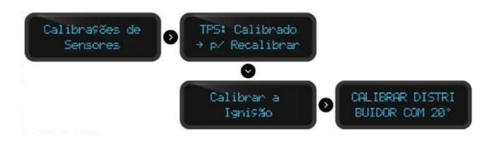
**Note**: When configured as a distributor, you should calibrate the window size before calibrating the ignition; if this calibration is not made, may happen a divergence at the ignition point.
