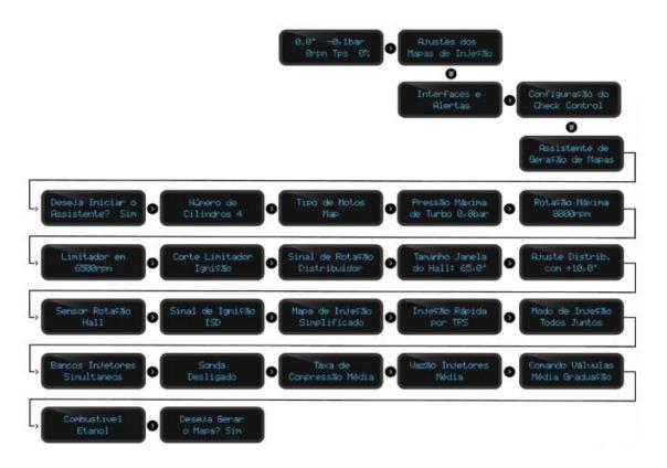
Right after the "Do you want to generate the map?" field, the "Cfg. In/ Outputs" appears on the screen, so we have the possibility to configure the inputs and outputs in "Default" or "Custom" mode. The next screen asks for confirmation of this option "Generate Cfg. In/Outputs?", and then if you choose "Default" the setting will look like this:
