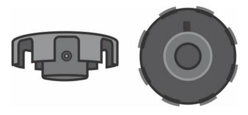
5- Alignment of the table relative to the sensor is very important. This joint is responsible for engine ignition point and fuel injection in the right moment, so is necessary that this "window" is on average 1mm greater than one of the other sides for the module has TDC reference of cylinder 01. (Choose the side that will pass through the sensor to remove material).
