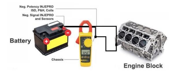
Must consider the total current consumption at startup and not only of the starter engine.
