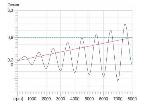
Example of a sine wave of an inductive sensor and low and high reference tensions.
