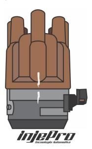
4- Unmount the distributor and create a mobile table relative to the distributor axis, this will allow the ideal adjustment of the ignition point without change the distributor position and the rotor position relative to the distributor cover.
